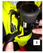
Continue feeding the hose into the inner pocket (Figure 3). Until the majority of the hose is positioned inside the pocket (Figure 4)
