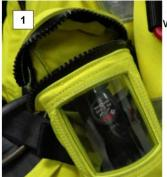
Insert the HUEBA all the way into the pocket, such that the gauge is visible through the window. (Figure 1). This may cause the hose directly behind the first stage regulator to curl up (Figure 2)
