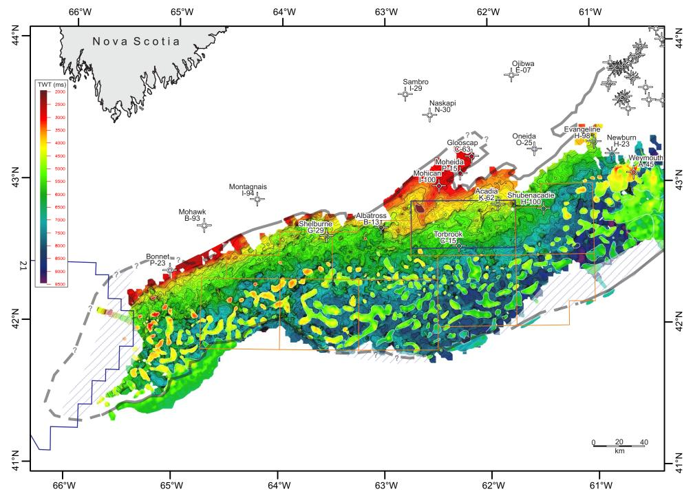
**Figure 13b** – Gridded time-structure map on the top autochthonous salt surface, overlain by the gridded surface from the top allochthonous salt bodies located predominantly in the ASM province. Autochthonous salt highs produce a polygonal network of minibasins in the DM province, many of which form the stems of overlying salt bodies.
