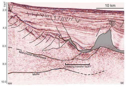
**Figure 10** – Close-up seismic profile of middle parts of Figure 2 (SD to proximal DM province), showing prominent northwest-dipping faults that may detach in a mid-crustal detachment surface. Slow water column velocities were depth converted, but remaining section is in TWT.
