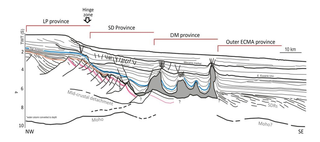
**Figure 2** – Line drawing of a composite seismic profile extending from the LaHave Platform (LP), across the Slope Detachment (SD) and Diapir and Minibasin (DM) provinces, and terminating in the Outer ECMA province where Seaward Dipping Reflections (SDRs) are recognized. Water column was depth converted, but remaining section is in two-way travel time. See Figure 1a for location.
