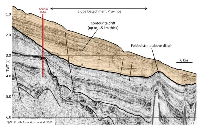
**Figure 18** – Northwest- to southeast-oriented profile across a thick contourite drift that is thickest above the SD province. Aggradation of this drift may have prompted down-slope squeezing of pre-existing salt diapirs in the ASM province. Profile from Kidston et al., (2005).
