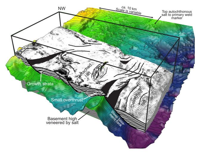
Figure 14 – Rafted blocks detaching above high-relief basement blocks veneered with autochthonous salt.
