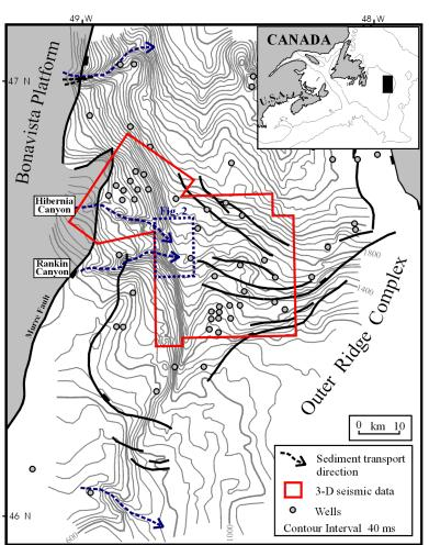
**Figure 1:** Location of Jeanne d'Arc Basin (inset) and contoured timestructure map on the Early Paleocene unconformity using a 2-4 km grid of 2-D migrated multi-channel seismic data. Also shown are the Early Paleocene sediment transport directions, the location of 3-D seismic data available in this study, and the location of figure 2.
