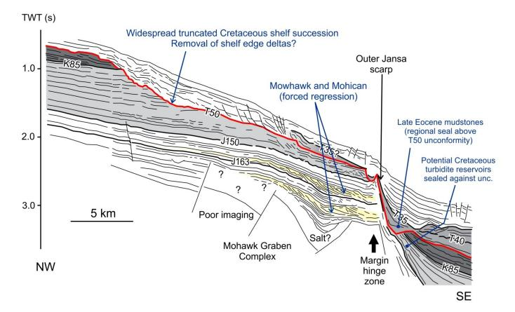
**Figure 2.15** Seismic profile line drawing from the outer part of the LaHave Platform, seaward of Mohawk B-93, showing widespread erosion along the T50 marker (red) and potential for an unconformity trap developed where Late Eocene shales drape the T50 truncation surface. Note also two intervals of progradation (interpreted as forced regressions) that probably delivered sand to the Jurassic slope.
