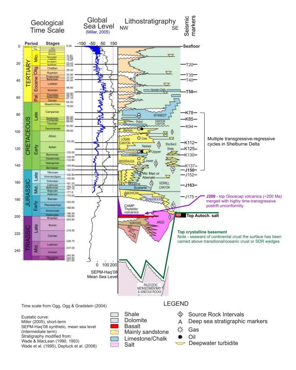
Figure 1.2 Stratigraphic column adpated from OETR (2011), with key seismic markers.
