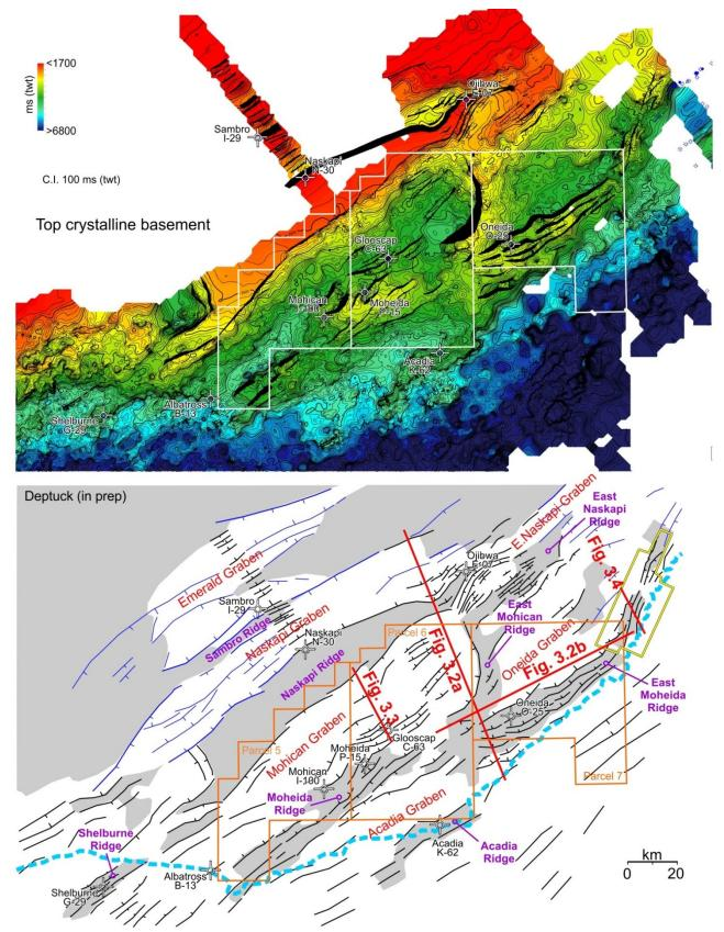
**Figure 3.1**. a) Time-structure map of the top of crystalline basement in the Central region. b) Corresponding map showing important basement elements. Faults in blue are from Wade and MacLean (1990). Line locations shown in red. Blue dashed line shows the overlying Upper Jurassic carbonate bank edge. \*Note that in (a) the water column was depth converted, removing the associated velocity sag caused by increasing water depths, particularly seaward of the modern shelf edge.
