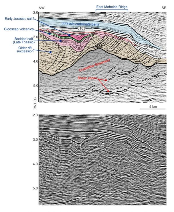
**Figure 3.4.** Uninterpreted and interpreted profile from the Blueberry 3D survey (CNSOPB program number NS24-E043-004E) across the seaward margin of the Oneida Graben and the East Moheida Ridge. The ridge is comprised of an elevated basement element veneered by a complexly faulted synrift succession. See Figure 3.1 for line location.
