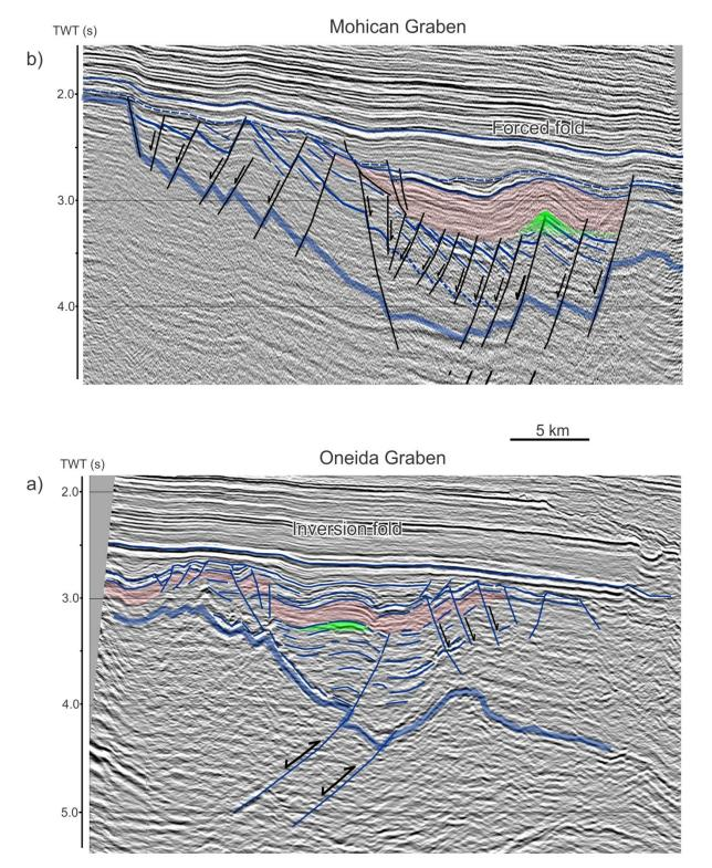
**Figure 3.7** Potential pre-salt traps involving synrift fluvial-lacustrine reservoirs draped by bedded salt; a) Synrift reservoirs incorporated into inversion folds and sealed by Late Triassic bedded salt; b) Synrift reservoirs sealed by a forced fold composed of Late Triassic bedded salt.
