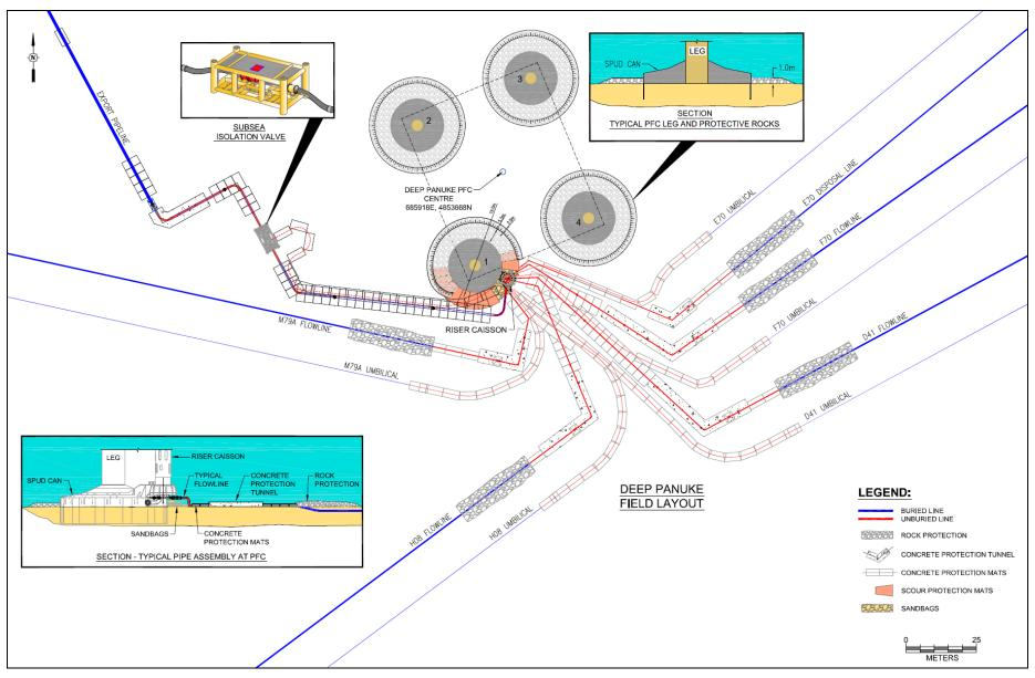
Figure 1.3 Deep Panuke Subsea Production Structures - PFC Area (From Offshore Production EEMP, May 21 2011)
