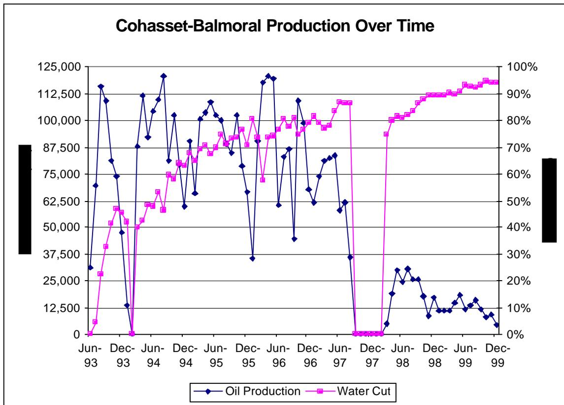
Most wells produced from several different zones commingled in the wellbore. In general, reservoir pressure support from the aquifer was excellent, and water injection for pressure maintenance was not required. All wells were ultimately produced to high water-cuts with electric submersible pumps.
