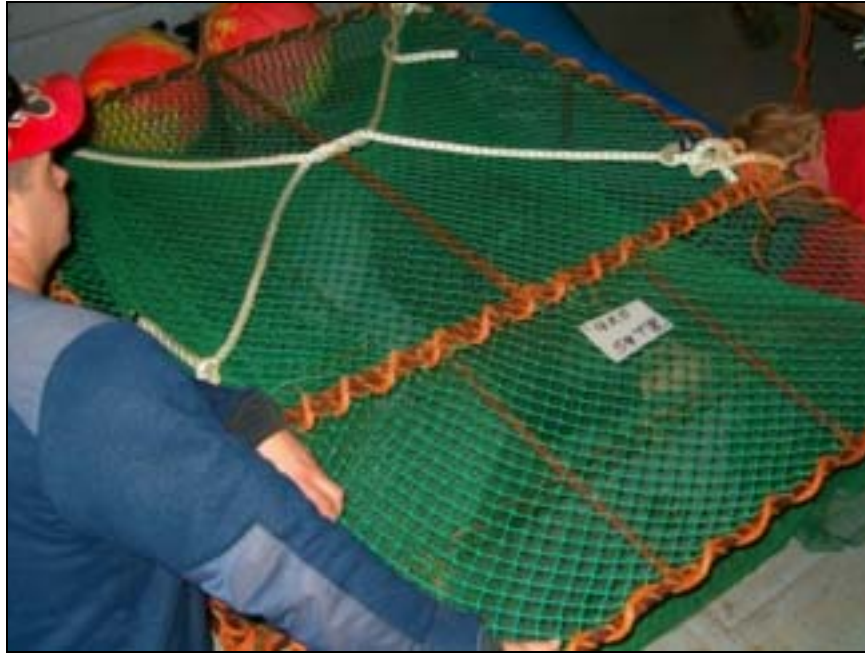
Photo 1: Fine Mesh Netting Was Installed Inside A Steel Framed Rectangular Crab Trap
