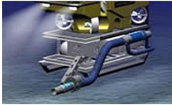
Figure 3.1 Schematic of ROV-Mounted Suction Pump
